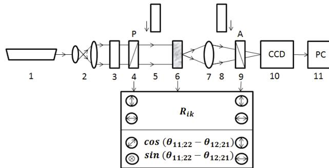
Figure. 1. The optical scheme of the polarimeter, where 1 - He-Ne laser; 2 - collimator; 3 - stationary quarter-wave plate; 5, 8 - mechanical movable quarter-wave plates; 4, 9 - polarizer and analyzer, respectively; 6 - the object of study; (b) 7 - micro lens; 10 - CCD camera; 11 - personal computer
