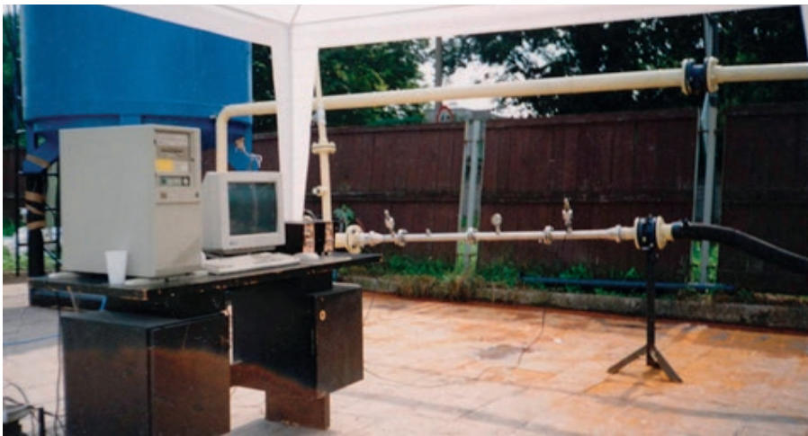
Fig. 2. Experimental stand for hydrodynamic cavitation
