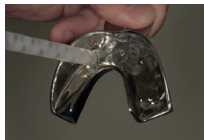
Fig. 3. EXACLEAR™ clear PVS material syringed onto a non-perforated mandibular tray to capture an accurate impression of the printed resin model.
