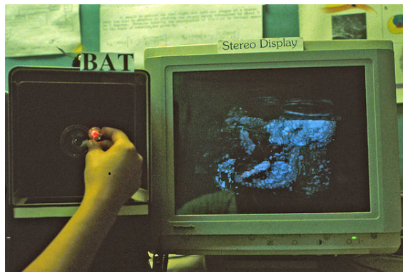
The NBRF “Bat,” a 3-D mouse (left) used for interacting with stereo images (right).
