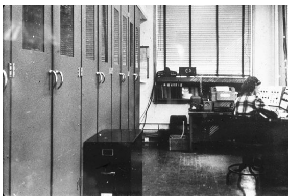
Terry Ledley operating the Standards Eastern Automatic Computer (SEAC) at the National Bureau of Standards in the early 1950s. Robert Ledley learned to program on this computer, first via paper tapes Terry brought to him and then by using the machine extensively himself.
