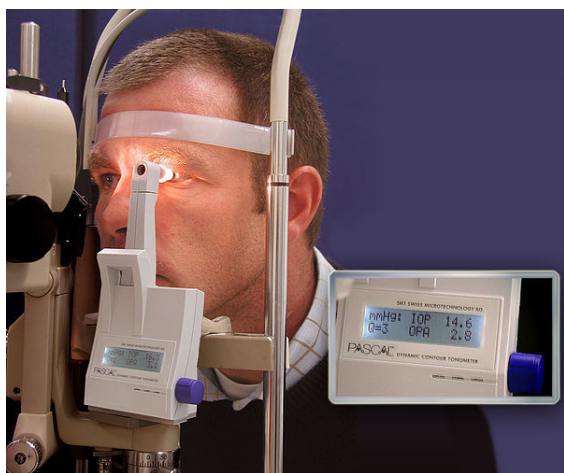
The PASCAL Dynamic Contour Tonometer. A monitor for detection of increased intraocular pressure.
