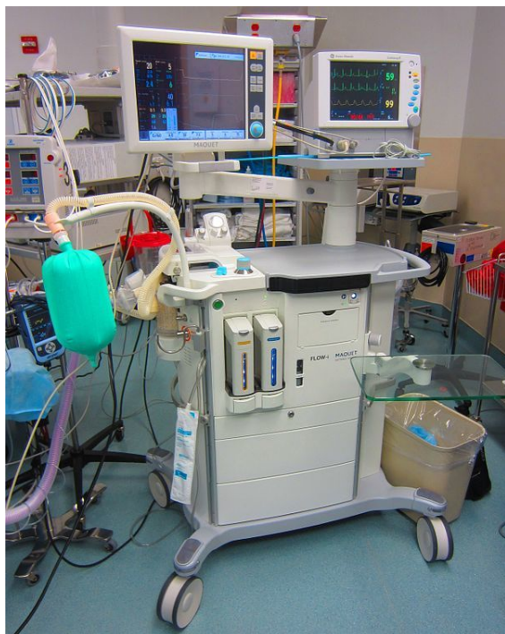
An anesthetic machine with integrated systems for monitoring of several vital parameters, including blood pressure and heart rate.
