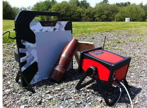
EOD training and material testing. A 105 mm shell is radiographed with battery powered portable X-ray generator and flat panel detector.
