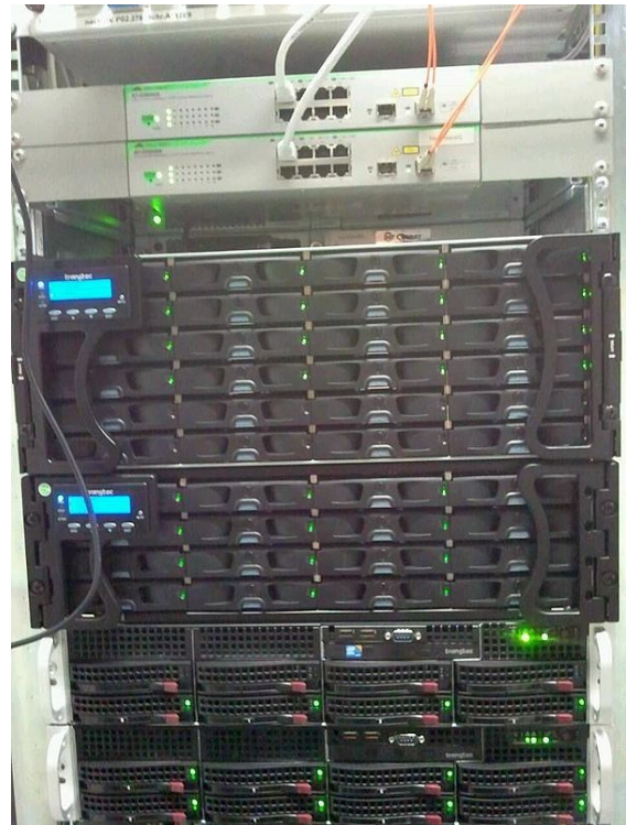
PACS-Server with 35 Terabyte RAID Archive and high speed fiber optic switch
